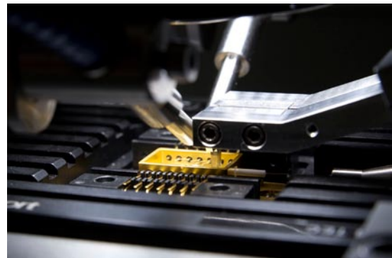
Fiber alignment in butterfly type packaging
